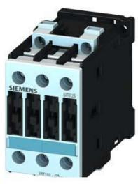
CONTACTOR, AC-3 11 KW/400 V, AC 230 V, 50 HZ, 3-POLE, SIZE S0, SCREW CONNECTION
